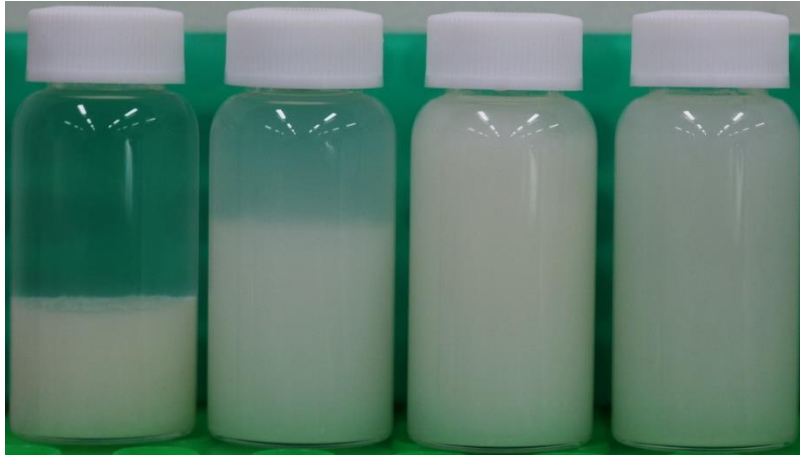
Fig. 1. Supermasscolloider (SM)-treated okara in water after 24 h. (A) 2% untreated; (B) 1% SM-treated; (C) 2% SM-treated; (D) 3% SM-treated.
