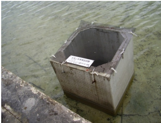
Photo. 1: Culture vessel fixed by anchor bolt set on Nishihama seashore in KUROSHIMA island for ocean seawater
