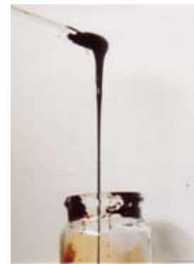
Crude oil-like product generated by thermal treatment of algal biomass
