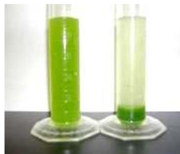
Cell harvesting by pH regulation
