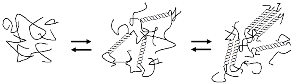
Fig. 2. Network formation of carrageenan polysaccharides
