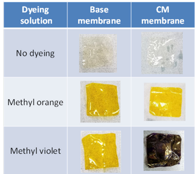
Fig. 7. Photos of base membrane (FAS-30) and prepared CM membrane before and after dyeing using methyl orange and methyl violet.
