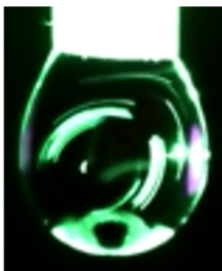
Fig. 1. Convection in droplet under microwave irradiation
