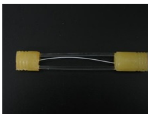
Figure 3. Photograph of the hollow fiber membrane module prepared in this study
