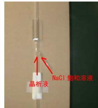
Fig. 8 Sampling tube with injecting branch for high crystal concentration
