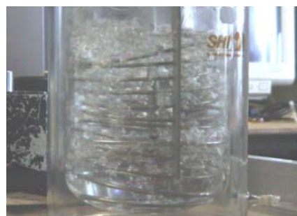
Fig. 2 Crystallization using a heating coil (before nucleation)
