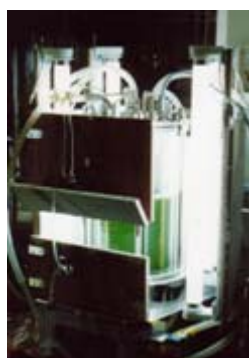
Photobioreactor for algal biomass production
