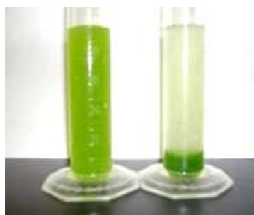
Cell harvesting by pH regulation
