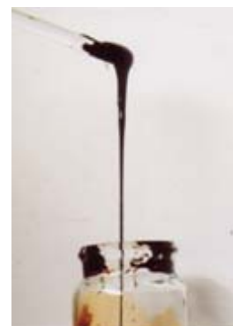
Crude oil-like product generated by thermal treatment of algal biomass
