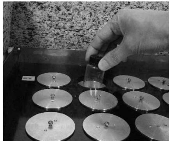
Fig. 3 Loading a sample to the calorimeter.
