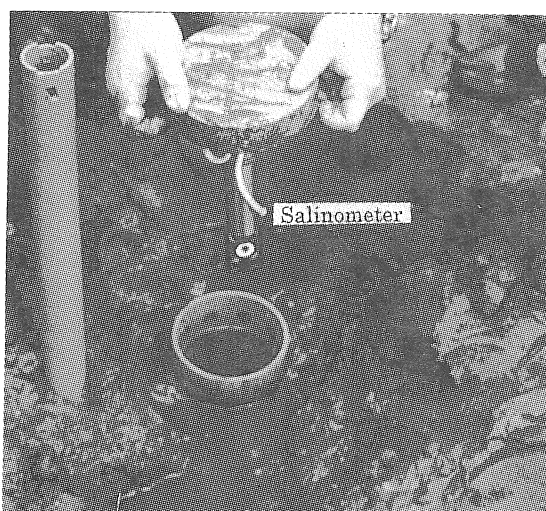
Fig. 2 Salinometer being installed in the vinyl chloride pipe in soil (July 3, 1999).
