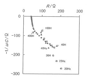
Cole-Cole plot of the impedance for the bed of Na-type cationic ion-exchange resin
